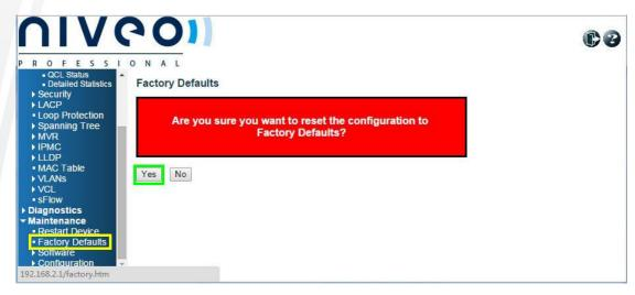
As shown in the figure above, choose **Maintenance** -> **Factory Defaults**, then click **Yes**, the switch will reset its configuration to factory defaults. Once the resetting finished, the switch will give a report as below:
