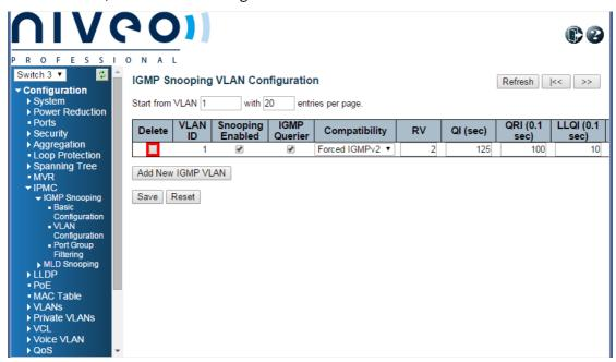
As shown in the figure above, a checkbox appears in the **Delete** cell, and other configuration items are the same as what we configured ago.
