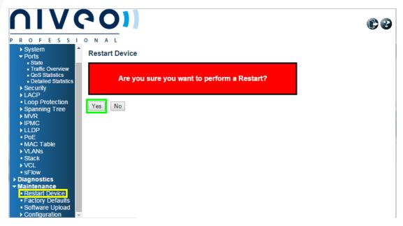
As shown in the figure above, choose **Maintenance** -> **Restart Device**, then click **Yes**. The switch will reboot to activate the stack feature.
