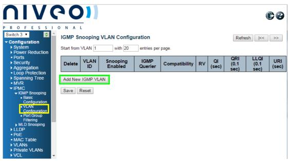
As shown in the figure above, choose **Configuration** -> **IPMC** -> **IGMP Snooping** -> **VLAN Configuration**, click **Add New IGMP VLAN**, then operate as below.
