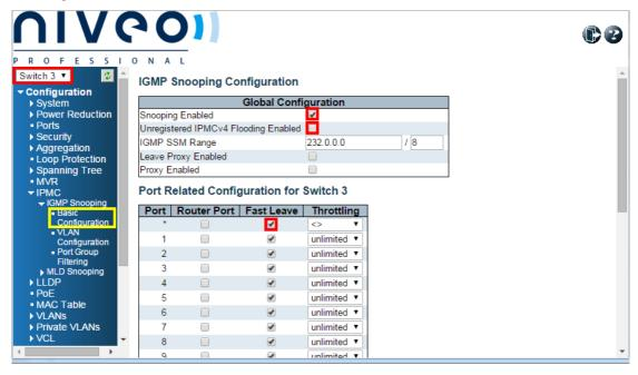
As shown in the figure above, choose **Configuration** -> **IPMC** -> **IGMP Snooping** -> **Basic Configuration**, then operate as below.
