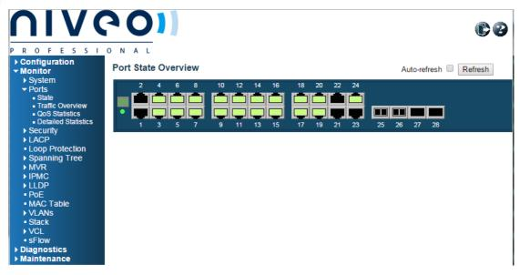
As shown in the above figure, after you log in to a Niveo NGSM24G4S switch which is not in a stack, there is only one switch in the **port state overview** page. To enable the stack feature, please operate as following steps:
