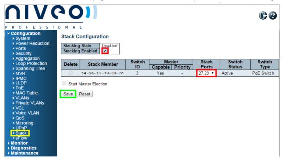
As shown in the figure above, choose **Configuration** -> **Stack**, configure as below:
