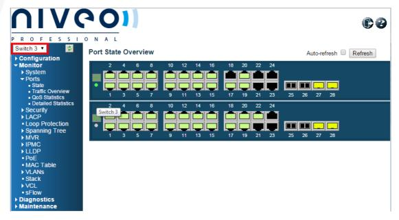
As shown in the above figure, all switches in the stack can be seen in the **Port State Overview** page. Furthermore, at the top left corner, the web server shows a dropdown list which include all stacked switches. In some configuration pages, by this list, you can choose different switch as current operation object.
