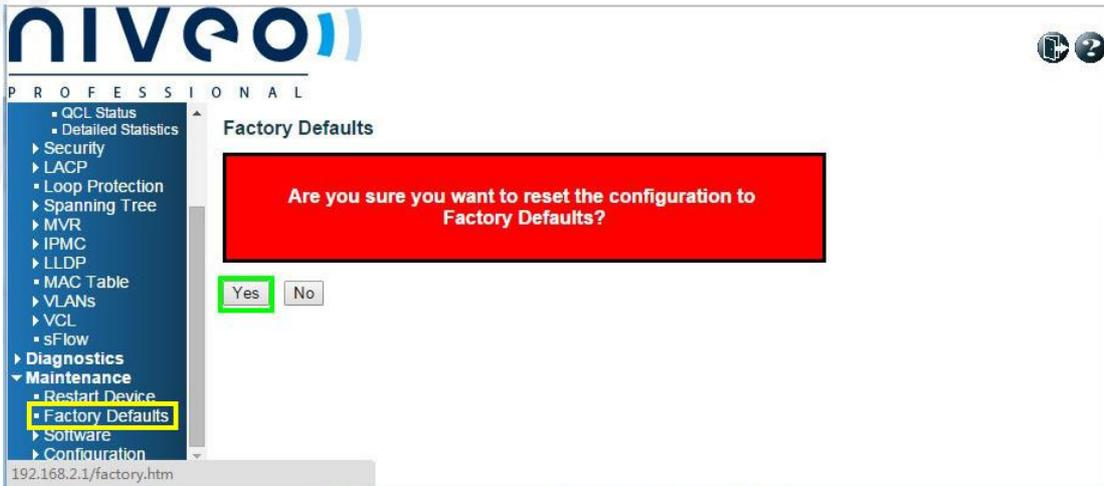
As shown in the figure above, choose **Maintenance** -> **Factory Defaults**, then click **Yes**, the switch will reset its configuration to factory defaults. Once the resetting finished, the switch will give a report as below:
